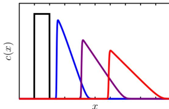
Figure: Persisting shock at tail, development of rarefaction wave at front
